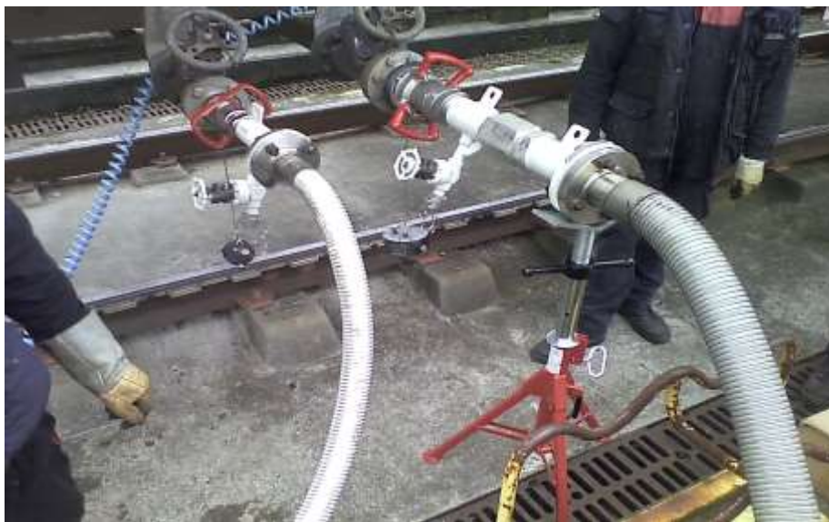
Figure 9: Example of connector (dry disconnect coupling to flange, mounted to unloading arm)
