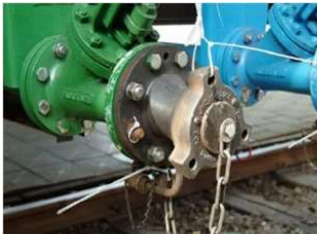
Figure 6: example of WECO connection mounted on flange.
