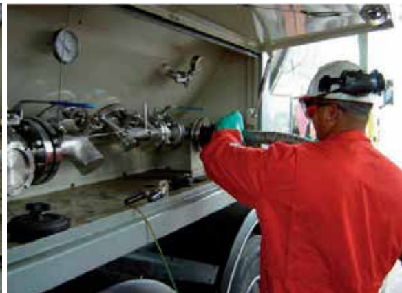
Fig. 4/5 Worker in protective clothing, connecting DDC liquid connection
