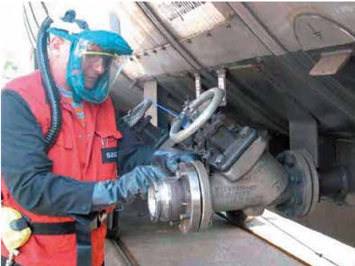
Fig. 10 Fully protected operator checking for a spill
