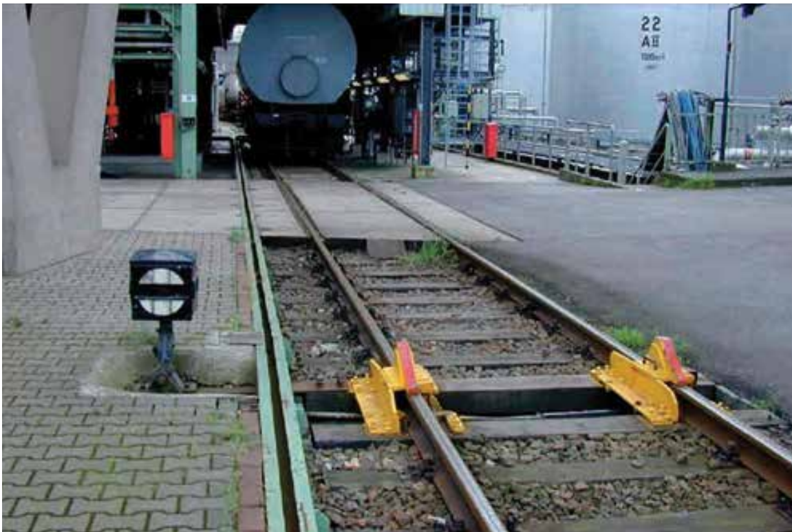
Fig. 6 Derailer at a filling station to prevent other railcars from entering the loading station
