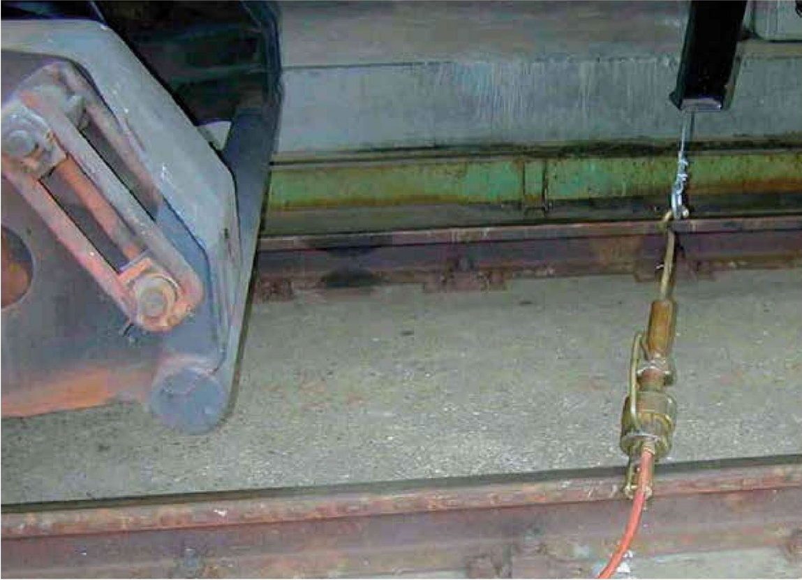
Fig. 9 Rail hook combined with a remote control, which closes the bottom valve if activated. This example shows only the set up for liquefied gas railcars.
